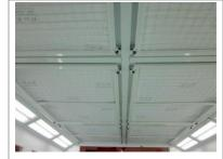
The filtering ceiling is formed by a bearing structure made of a sequence of plane trusses of section bars, in which inside part are mounted the filtering panels, covered with white coloured frames fixed with special Bakelite pommels.
