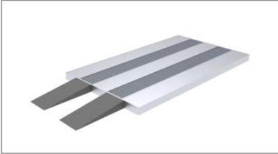
The metal basement (h.300 mm) is endowed with modular panels of electro galvanized grades (two lines grill and three lines checkered plate) forged to industrial sweater in designed to withstand heavy weight equipment with maximum weight to be supported of 650 Kg for wheel print. Besides, there are several under-grates metallic looms in order to close central zones where suction is not provided, with paint-stop filter.
