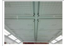
The filtering ceiling is formed by a bearing structure made of a sequence of plane trusses of section bars, in which inside part are mounted the filtering panels, covered with white coloured frames fixed with special Bakelite pommels.
