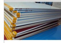
Sandwich panels of 50 mm thick, specifically built by BZB, assembled together by means of a male-female system, without welds or screws, with internal **EPS** insulation of 50 Kg/m³ density, closed around its perimeter.
